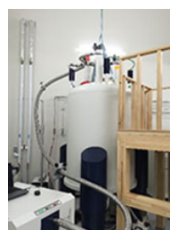
800 MHz superconducting nuclear magnetic resonance equipment
