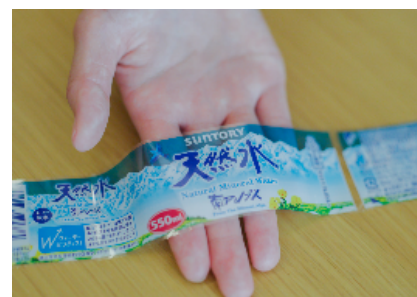
12 \mu\text{m} thick roll label, thinnest in Japan
